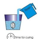
7. - Allow the resin to cure. Keep it warm if possible, cure in a well-ventilated area, and if possible, expose the resin to sunlight while it is curing.
